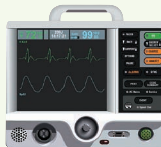
Figure 3: Portable defibrillator with CCFL backlight
