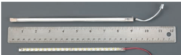
Figure 1: CCFLs have been the dominant backlighting technology for medical displays, but challenges from LED backlights (such as the LED rail shown here) are on the horizon.
