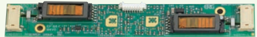
Figure 2: Smart Force inverters have been designed for display applications like portable defibrillators (Figure 3) that require high efficiency, wide range dimming, and lamp current stability over a wide input voltage range.
