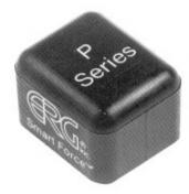
5, 6, 9, 12, 15, 18, 24, 28 Vdc standard -25°C to + 85°C standard (other ranges available)  $1.01'' \times .82'' \times .70''$  high  $25.3 \text{ mm} \times 20.5 \text{ mm} \times 17.5 \text{ mm}$  high PC mounting standard Plastic case standard All standard units fully encapsulated with epoxy resin
