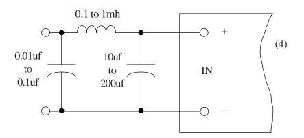
Typical Input Filter Configurations
