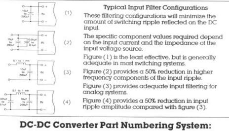
E - X X X - X X X - X Series 2 Digit Input Voltage Code Output Voltage 0 utput Voltage in 100 Volts Output Suffix (S) Single Output (D) Dual Output (U) Unregulated (R) Regulated (CT) Center Tapped
