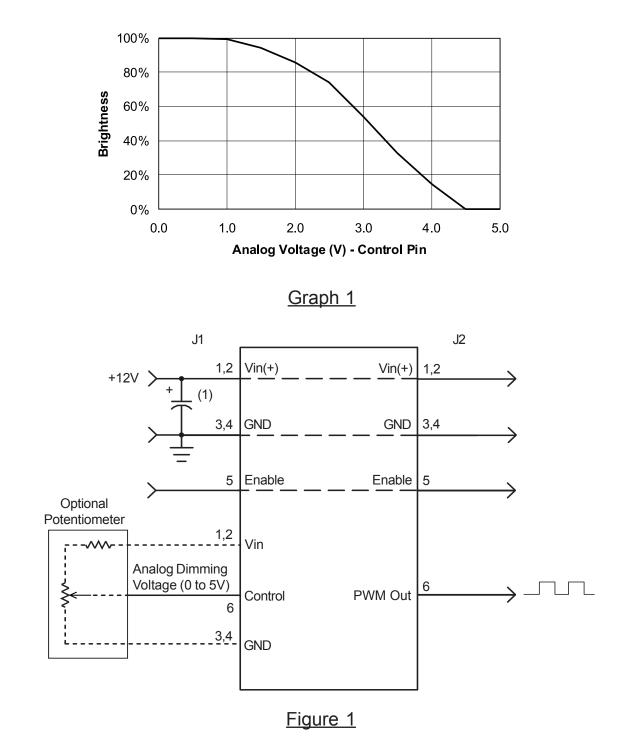
(1) Low ESR type input by-pass capacitor (10 uF - 220 uF) may be required to reduce reflected ripple and to improve power supply response.
